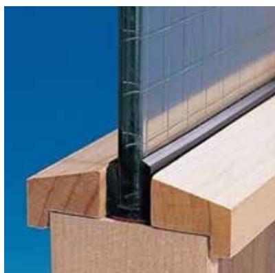
GLASS INTUMESCENT FIRE SEAL Intumescent glazing gasket
